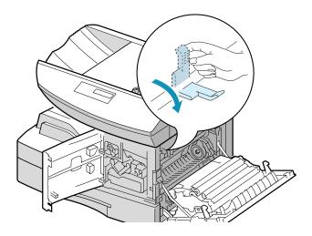
**4** Turn the jam remove lever in the direction of the arrow to move the paper to the exit area, then gently pull the paper out through the exit area.
